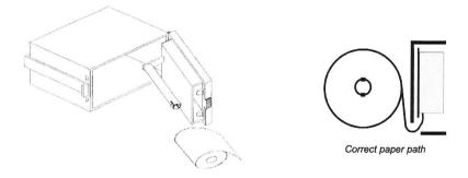
The printer incorporates an automatic paper feed facility. With a new paper roll mounted on the carrier and with a clean straight edge to the paper, present the paper to the entry point at the lower edge of the mechanism. The paper will be sensed by the mechanism and automatically feed through into a position ready for printing
